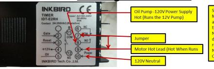
System uses Shredder Motor lead to initiate and control Oiling cycle through timing cycles Normally open closes during the "A" cycle to run the pump, returns to Normally Open during "B" Cycle, shutting off pump
